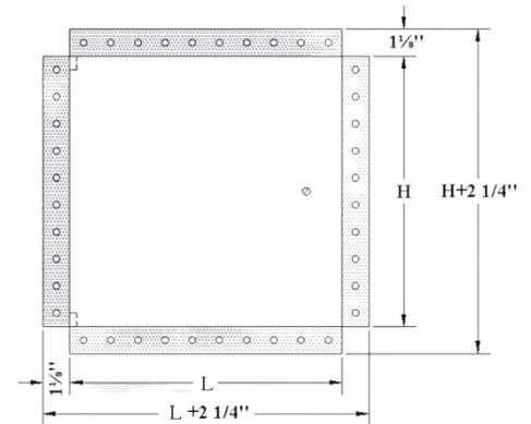
L'OUVERTURE DANS LE MUR = DIMENSIONS DE LA PORTE + 1/4 PO OU + 6 mm
