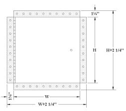
ROUGH WALL OPENING IS DOOR SIZE + 1/4" OR + 6MM \*NOT AVAILABLE FOR CEILING RATING (MAXIMUM 24"X36")
