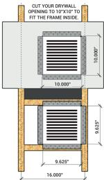
A premium flush mount exhaust fan cover for a 10" x 10" drywall opening. This cover can also be used as a cold air return, and yields a 8.125"x8.125" accessible area.
