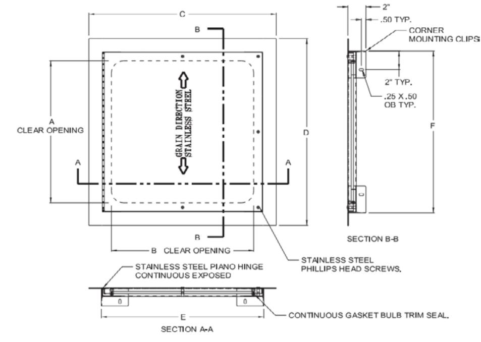
THIS DOOR HAS BEEN TESTED AS FOLLOWS: AIR INFILTRATION: LESS THAN 0.01 CFM/SQ FOOT: ASTM E 283 WATER RESISTANCE: NO LEAKAGE AT 15.05 PSF: ASTM E 331 STANDARD FEATURES: FRAME FULLY WELDED TO PREVENT LEAKAGE. CONTINUOUS GASKET BULB TRIM SEAL. STAINLESS STEEL PHILLIPS HEAD SCREWS
