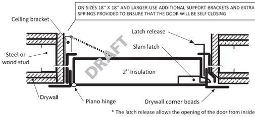
\* The latch release allows the opening of the door from inside.
